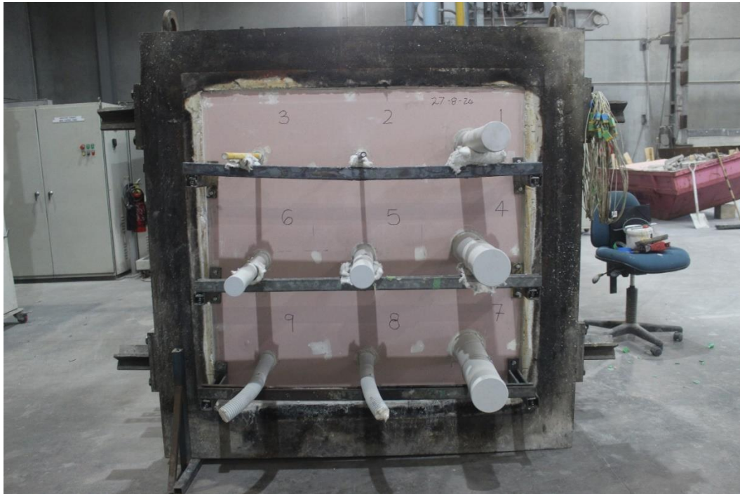
Figure 1 – Exposed face prior to test commencement
